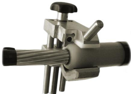
The chamfering tool is suitable for XLPE cable insulation for a range of diameter from 15 mm to 60 mm. This very simple to handle tool removes sharp edges at the cut-off edge of cable insulation to avoid possible damage to and to ease installation of slip-on accessories.
