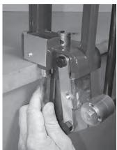
**Install** spent primer tube. Leave the cap on the tube if you are not routing to a trashcan.
