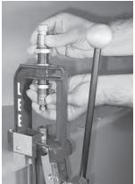
To prevent this be sure to tighten the lock rings only when the lock pin is in the groove of the Quick-change insert. If your press is in a humid climate lube the bushing and frame threads to prevent corrosion.
