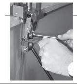
The toggle linkage operates on special aircraft type full body bolts and is retained with a crown lock nut. You can adjust the lock nut to eliminate any side play in the linkage.
