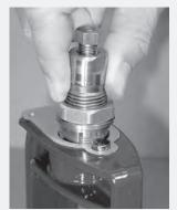
Insert the holder into the press Remove the die by depressdie in or out for proper operation. change to your next die.
