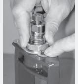
so that the lock groove will line ing the lock button and rotate up when secured. Adjust your the die ½ of a turn lift out and
