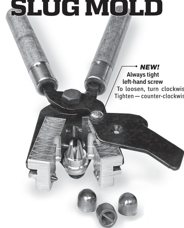
The Lee Slug Mold incorporates the exclusive "Drive Key" (patent rights reserved). The Drive Key doubles as an internal support for the wad. This eliminates the need to fill the base of the slug or require nitro cards in the shot cup. The Drive Key assures positive rotation of the slug in rifled barrels.
