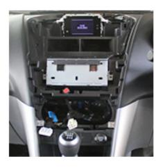
4. Unclip the plastic panel from around the OEM display and insert into the supplied facia panel.
