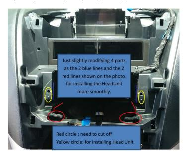
7. Take off the retaining clips from the OEM panel and insert into the supplied facia. Clip the supplied facia into place over the aftermarket head unit to complete the installation.
