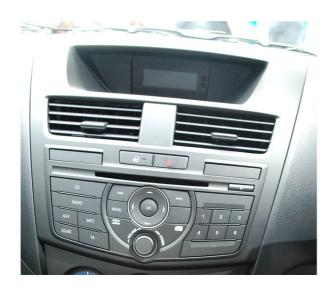
2. Unclip the air vents from the OEM panel and insert into the supplied facia.
