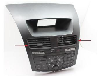
3. Remove the OEM head unit by removing the screws on the left and right hand side.
