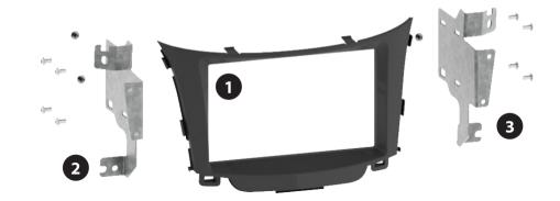
Place double DIN head unit and fix it. Place facia plate.
