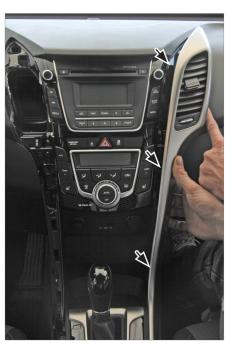
Remove side panels with air vents at left and right side (see arrows)
