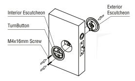
**Test by rotating turnbutton** - if the operation is not smooth, loosen screws and re-adjust the escutcheon positions
