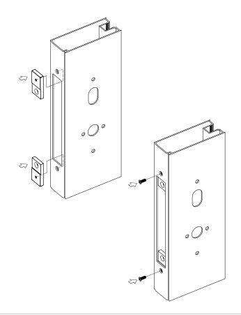
3. Install mortice lock with screws provided
