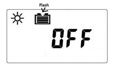
DC as Priority Source; Displays a flashing Battery Icon & OFF
