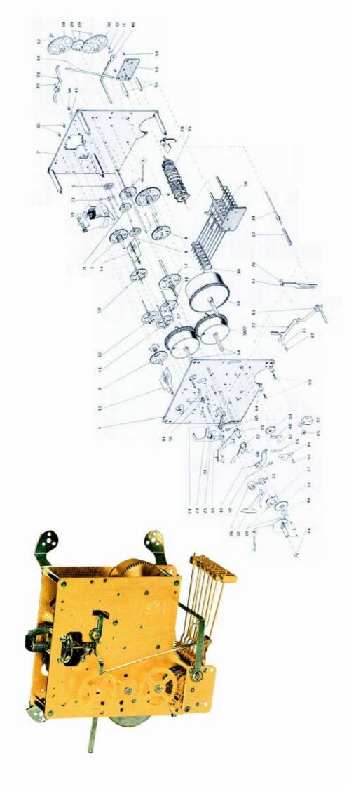
8 DAY SPRING WOUND TRIPLE CHIME / FLOATING BALANCE MOVEMENT Eight chime hammers strike a steel rod chime assembly (bottom mounted) Hand shaft length 33.1 mm. Plate size 120 mm x 120 mm 4 front mounting legs W1050.020
