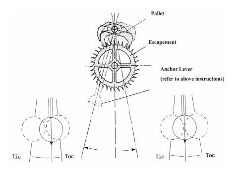
**Note**: After performing this adjustment the distance from the center to the **TIC** should be the same as the distance from the center to the **TOC**.
