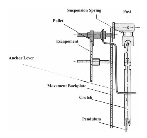
**Note**: A correctly adjusted movement will run smoothly and continuously, producing a balanced and familiar sound. Poorly adjusted movements seldom run for very long and produce notably different sounds.
