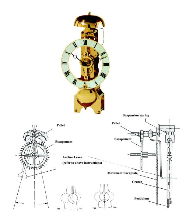
A smooth and balanced pendulum swing will generate an even TIC TOC sound, (50% Tic - 50% Toc) If the swing is not balanced (70% Tic - 30% Toc) the clock will eventually slow and stop. Listen carefully when performing set up.
