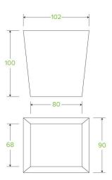
BioBoard Noodle Boxes are made from sustainably sourced  $FSC^{\mathbb{M}}$  Mix certified paperboard and lined with waterproof  $Ingeo^{\mathbb{M}}$  – a bioplastic product made from plants, not oil. This 26oz noodle box is printed kraftlook. Certified industrially compostable to AS4736.
