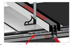
There should be a gap between the position indicator lens and the ruler on the main tube.
