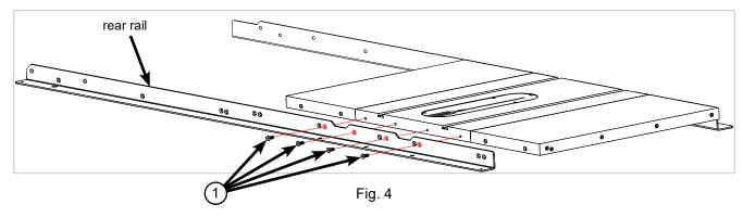
5. Finish mounting the rear rail to your saw by inserting an M8 x 25 countersunk socket head bolt through the open hole at the end of each extension wing (see Fig. 5a), and placing an M8 washer, an M8 lock washer, and an M8 hex nut on the threaded end of each bolt (see Fig. 5b). Hand tighten the nuts; do not fully tighten them.
