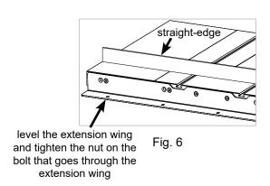
7. Once the rails are in place you can mount the extension table to the rails. The hardware needed to mount the extension table to the rails is in the T-Glide Table Hardware Pack shown below.
