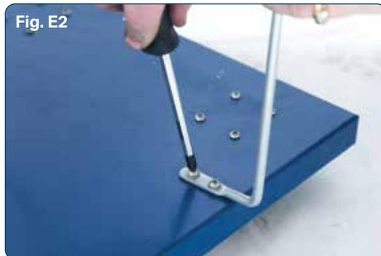
4. Attach the upper bag support to the collector using the two M4-7 x 8 Phillips head screws.
