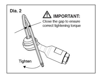
IMPORTANT: Ensure bolt is correctly tightened with the lan Key. Stop tightening the screw when gap on the lan key is closed (see Diagram 2).
