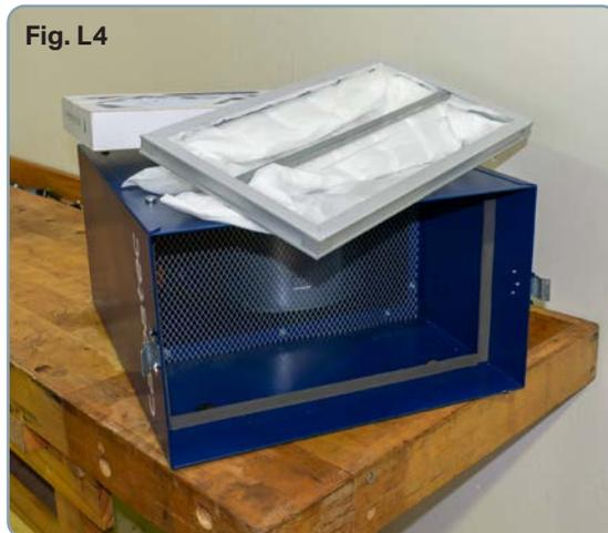
**NOTE:** There is an arrow indicating the air flow direction on the outer filter. Make sure the filter is inserted facing the proper direction.
