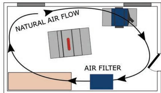
3. When an air filter is placed too close to any obstructions, such as walls, much of the room will be unfiltered as circulation is diminished when the velocity of the air is lost. There must be a clearance of at least 1m from any obstructions in front or at the back of the unit.
