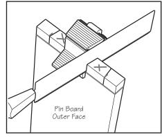
Figure 14: Cutting the pins.
