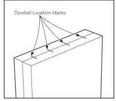
Figure 6: Mark out locations of dovetail cuts. Mark across both boards at once with a single mark at each location.
