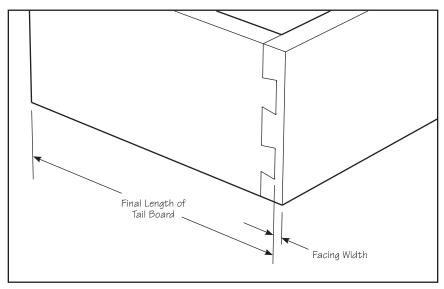
Figure 20: Half-blind dovetail joint.
