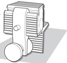
Figure 13: Dovetail saw guide set to cut pins. Note that taper is horizontal.
