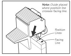
Figure 24: Guide located for cutting pins.
