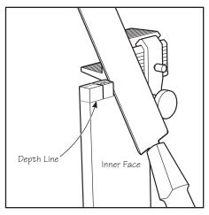
Figure 25: Cutting the pins. Note the angle of the saw.
