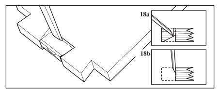
Figure 18: Cutting the final depth of the dovetail.
