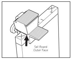
Figure 10: Guide in place; note that waste area is exposed and guide is exactly on the mark.
