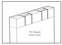
Figure 26: Pin board after the cuts have been made.
