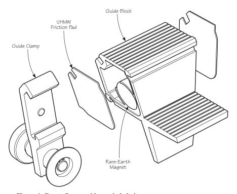
Figure 1: Dovetail saw guide, exploded view.
