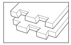
Figure 19: Finished pin and tail boards.
