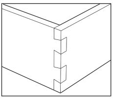
Figure 2: Typical full dovetail joint.
