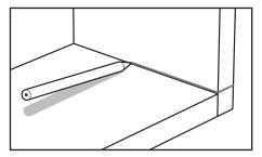
Figure 8: Marking the depth of the dovetails.
