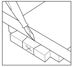
Figure 16: Scoring the depth of the dovetails.
