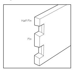
Figure 4: The pin board.
