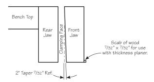
8. Insert the vise screw nuts into the back of the rear jaw, aligning them square. Using a 1/4" drill bit in the screw holes, lightly mark the centers. Before removing the nuts, mark both the orientation for realignment and the hole each came from. Remove
