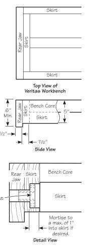
will be slightly reduced due to the thickness of the rear jaw assembly. If you wish, the nuts may be mortised into the skirt. Even if you don't mortise the nuts into the skirt, the twin-screw vise gives you ample capacity.
