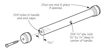
To assemble the speed knob, take one of your handles (right side if you are right handed) and drill a 17/64" hole through the center (see illustration at right).
