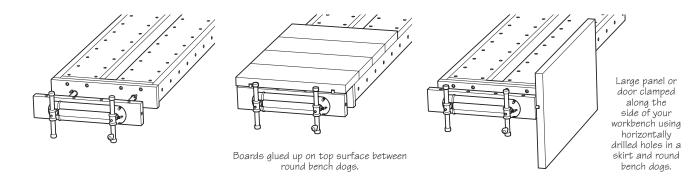
The Veritas Twin-Screw Vise is designed to enable you to skew the front jaw in either direction. By simply disengaging the spring-loaded drive/shear pin, you may turn either screw independently of the other to produce the required skew. For example, if you are gluing boards between bench dogs and one side closes up before the other, you can disengage the pin and turn one screw to compensate.
