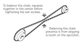
If after installing your chain you observe any sag, use one or two of the #10 wood screws and chain rollers to support the bottom of the chain. **Do not** install the spacer any higher than the bottom of the chain loop when taut.
