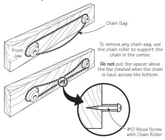
If there is a great amount of sag in your chain (more than half a link), the half link may be used. To determine if the half link can be used, there must be enough slack to fold the chain into the shape of the letter Z (see illustration).
