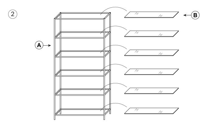
Gently place glass shelf (B) on to metal frame (A) fitted with bumper (C). **TIP:** Work from the top shelf down and support shelf from under side as you lower it carefully into frame.
