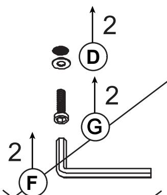
2 Attach dividers (C) to shelves (B) using washers (D), bolts (E) and allen key (F), as shown.
