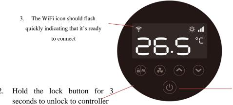
1. Hold the power button for 3 seconds
