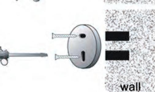
3.Put fixing block cover on the holes and fix firmly by expansion screws.
