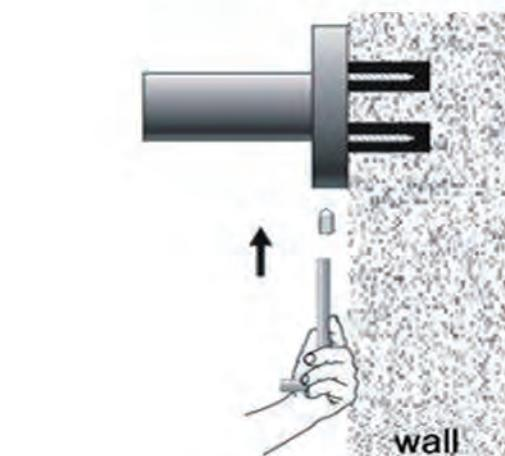
5. Screw grub screws into the base, make it against to the fixing block tight and firm.
