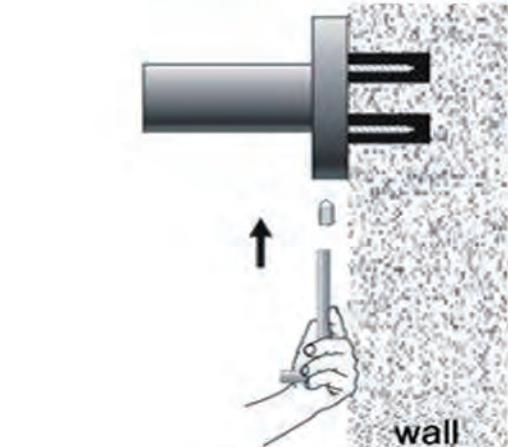
5. Screw grub screws into the base, make it against to the fixing block tight and firm.
