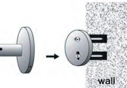
4. Put the base of bathroom accessory cover on the fixing blocks.
