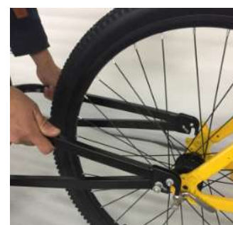
put assembled trailer on the quick release
