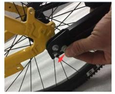
put down the safe lock and move down along the arrow sign
