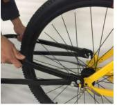
put assembled trailer on the quick release
