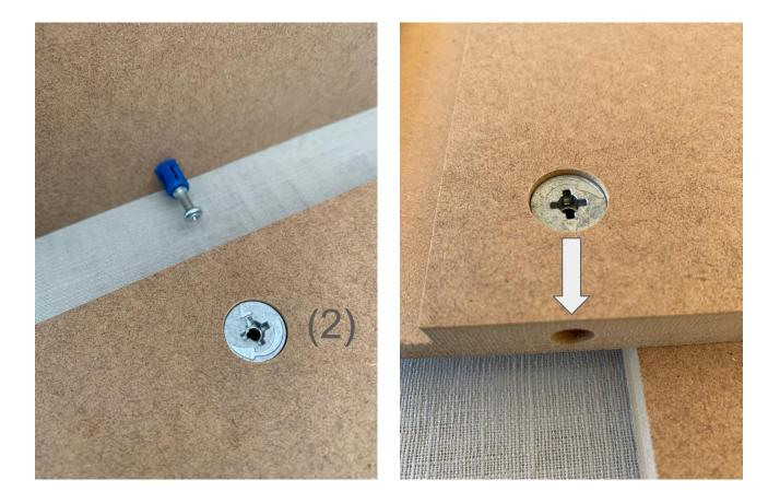
Fit cams (2) into holes, with the arrow on the cam pointing in the direction of the hole on the side. *Tools for the art of jewellery*
