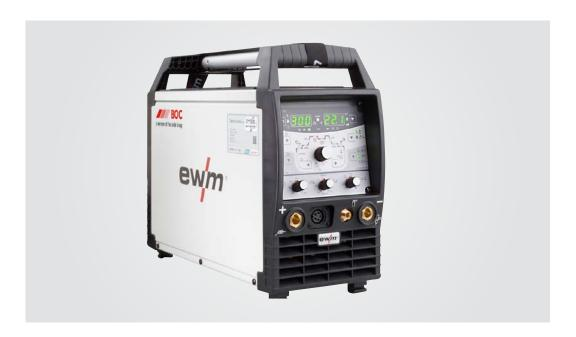
The *EWM Tetrix 300 ACDC* is an efficient and portable machine that is gas or optionally liquid-cooled with the *cool 40 U31* cooling unit that allows excellent torch cooling (available separately). Its MMA pulse welding capabilities includes adjustable hot start current, arc force and anti-stick functions. A special AC welding procedure with the machine allows the user the flexibility to join different aluminium plates together eg welding 1mm sheet to a 10mm plate.
