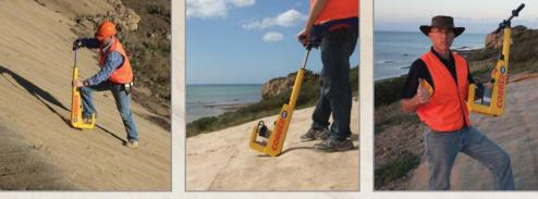
Available in two sizes, the **COBBER<sup>™</sup> 150** for 150 mm staples, and a **COBBER<sup>™</sup> 200** for 200 mm staples. Both are made from HD nail wire at an average of 900 Mpa.
