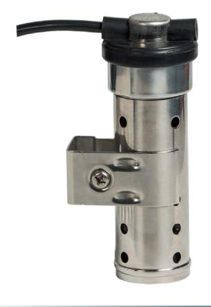
This device is for detecting water level at the bottom of your boat. When water comes up to alarm level, the buzzer will sound. The housing, which can be conveniently disassembled and cleaned, can prevent foreign particles from obstructing the movement of the float.
