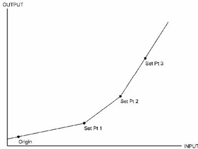
If an origin and 3 points had been programmed then between these points the output would follow the profile and the centre LED will flash about once per second. If the input goes past either the Origin or, in this case, Set Pt 3, the unit will extrapolate a linear output using the last gradient calculated and a 'o' ('o'ut of range) will appear in the display.
