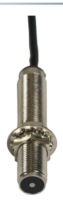
This sensor applies induction to measure the speed, and it has big output signal, good anti-interference, no need of amplification or external connection of power supply. It can be used under severe circumstances, such as, smog, oil, moisture, etc.
