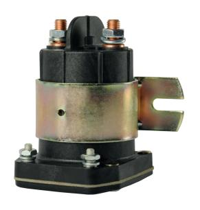
Designed for high current applications, the Trombetta 'Bear' range of solenoid contactors represent excellent value. The combination of high impact plastic and zinc steel housing provides a robust device, compact in size and easy to install. Available with either 12 or 24VDC coils and copper or long life silver alloy the 'Bear' is ideal for battery management, emergency starting, load switching and a myriad of demanding transport applications.
