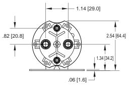
DIMENSIONS IN BRACKETS [] ARE MILLIMETERS
