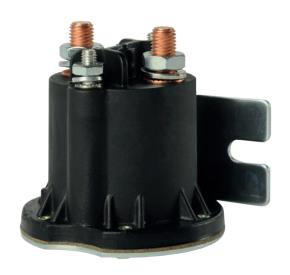
The Trombetta PowerSeal range features an environmentally sealed housing to IEC 60529, IP66 and IP67 standard. It is the first contactor designed specifically for electric vehicles and other applications where environmental protection is a must. The sealed design is the core of the construction and is optimized for high performance at lower cost. Constructed from high impact plastic with zinc plated steel frame, the PowerSeal range is designed for high performance, durability and longevity.
