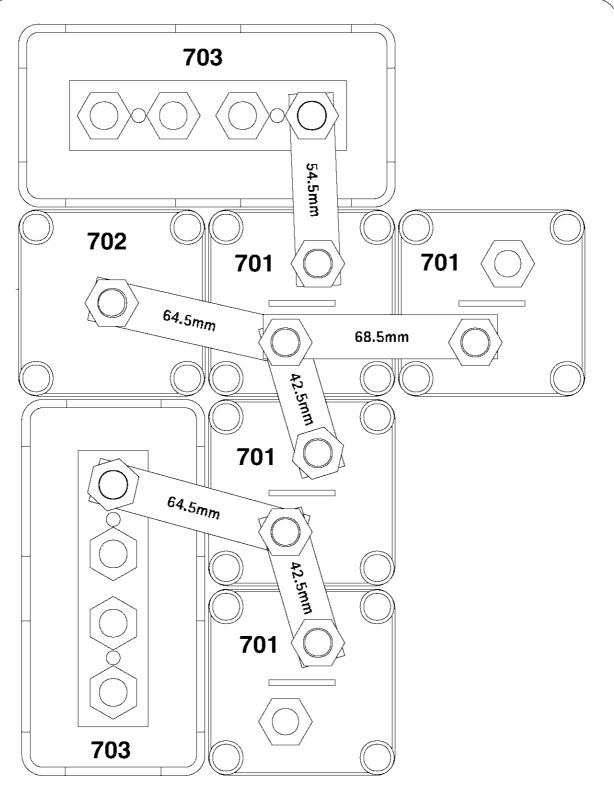
Diagram depicts typical Master Switch setup using 708 Terminal Links.
