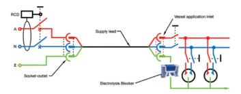
The Electrolysis Blocker shall be connected into the supply protective earthing conductor before it connects to the vessel's earth system. It should be installed where there is protection from accidental access, good ventilation, as close as practical to the shore power inlet / distribution panel and behind the appliance inlet. Use the mounting slots to secure it.
