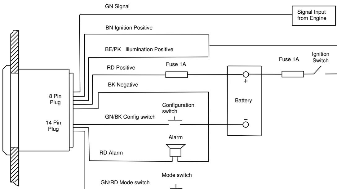
To calibrate the tachometer, the number of impulses per engine revolution must be programmed into the instrument.
