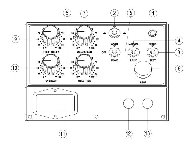
Power cord. Connect the power cord to 1 phase 100V~240VAC
