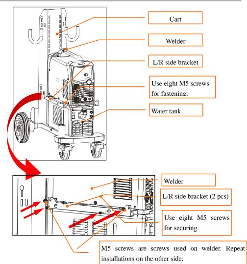
Step 6 Attach support brackets to welder.
