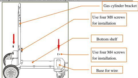
Step 2 Attach wire bracket to top shelf.
