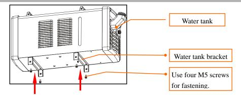
Step 4 Place water tank on bottom base and secure it in place.
