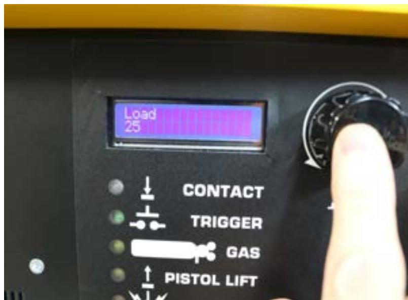
Then **PRESS & RELEASE** the control knob. This will load the saved parameter set into the current operating parameters. A double audible tone will sound and the display will return to the operating screen (now displaying the loaded parameters).
