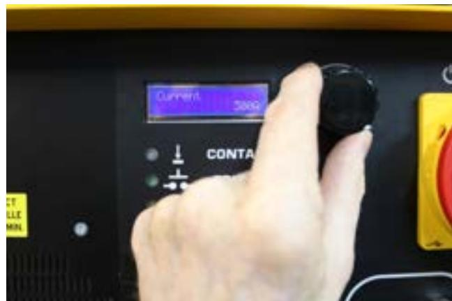
The next screen is to set the welding time (duration). The value is shown in milliseconds (mS) and is adjustable between 1mS and 1000mS.
