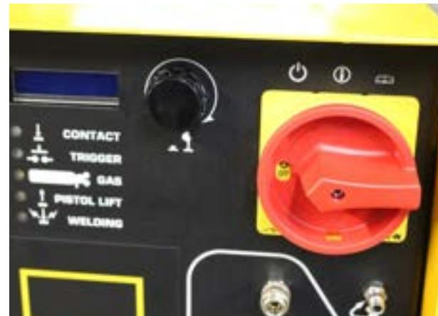
Plug the controller into a suitable three phase AC supply with a 100A motor rated fuse/breaker.
