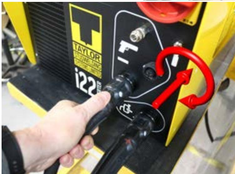
Plug the welding pistol cable into the controller. Note that the cable end weld plug has a peg which mates with the key slot in the panel mounted socket.
