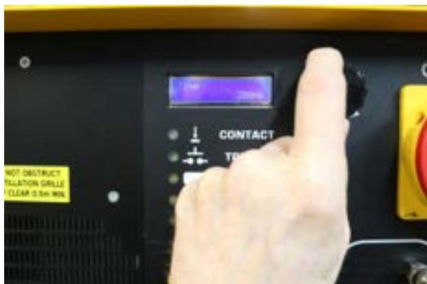
**TURN** the knob to set the required welding time. Once the desired number is reached.
