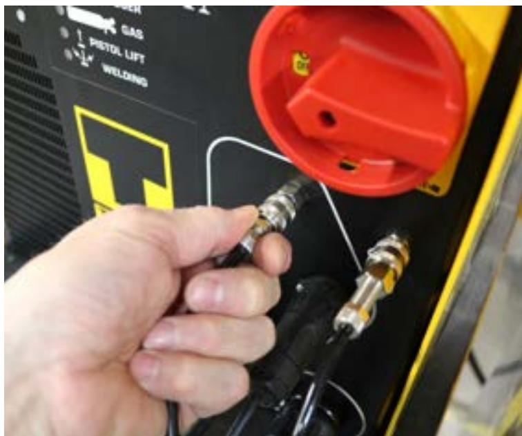
Connect the gas pipe from the pistol to the output socket on the front panel (optional).
