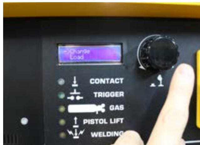
From this menu. You can elect to either "Change" the current welding parameters by adjusting the individual welding parameters or "Load" a previously saved parameter set from the controller memory.
