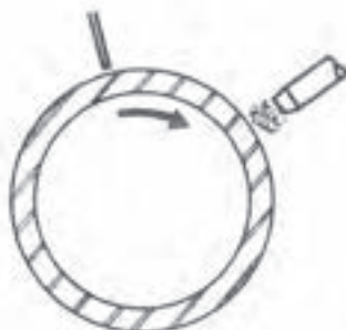
Figure 9 — Air applied to the work at the 2:30 o'clock position will cool both the work and the slag and aid slag removal.
