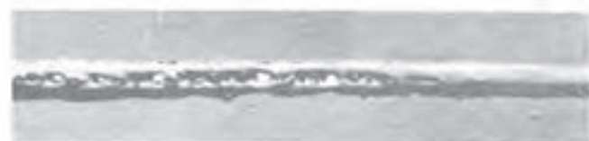
FIGURE 6 — Dirty flux can cause severe porosity.
