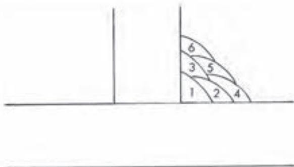
Figure 14 — Proper bead sequence for multiple pass fillets.
