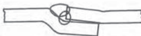
FIGURE 11 — Offset-lap welds inherently tend to trap flux in the bottom of the joint. First pass may be porous; second pass is sound.
