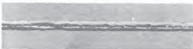
FIGURE 8 — Porosity from backward arc blow is more common on the finish end of welds in light gauge sheet metal than in any other type of weld.
