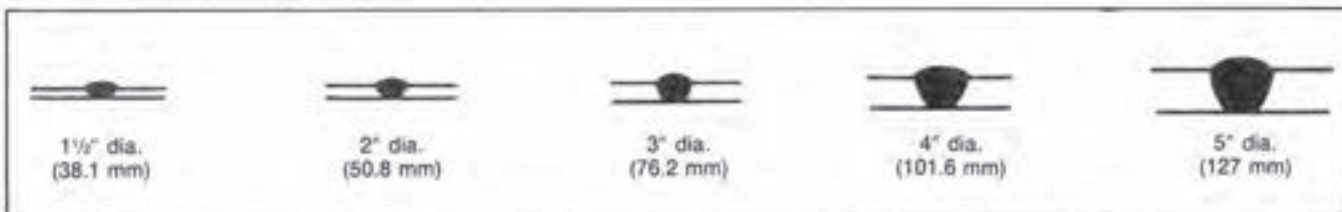
Figure 3 — Approximate size of the largest bead attainable on small diameters. To obtain these welds, backups are required on thin sections and special arrangements to prevent flux spilling may be necessary.
