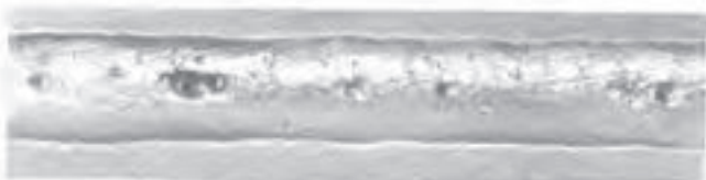
FIGURE 7 — Gas pockets in the weld results from insufficient flux coverage.
