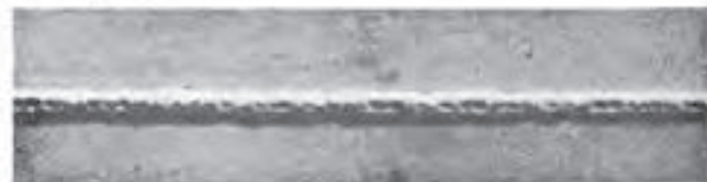
FIGURE 5 — Porosity caused by oily plate.
