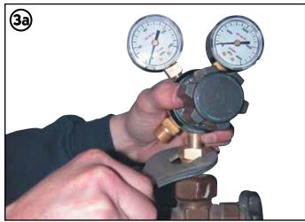
**3 - 3a.** Attach regulators to respective cylinders tighten using appropriate spanner supplied (note: black cylinder for oxygen and maroon cylinder for acetylene)
