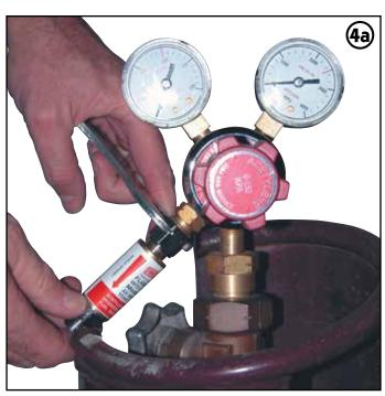
**4.** Connect approved **IBEDA** flash arrestors (AS4603 supplied) and tighten with appropriate spanner to regulators. **Note: These are colour coded and are thread orientated.**
