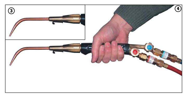
**4.** Adjust welding tip alignment by loosening mixer to correct the angle of the tip for operators safety and comfort and tighten mixer and **CHECK FOR LEAKS.**
