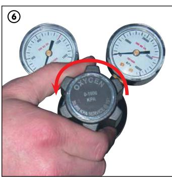
Before opening cylinder valves with regulators attached, **ENSURE** that regulator control knobs are fully wound in the **ANTI-CLOCKWISE** position.
