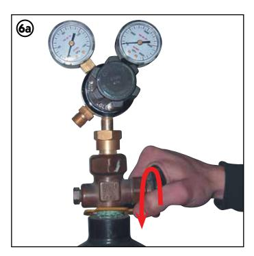
**6a. SLOWLY** open the cylinder valves so that high pressure gauge needle moves up gradually and check for leaks.
