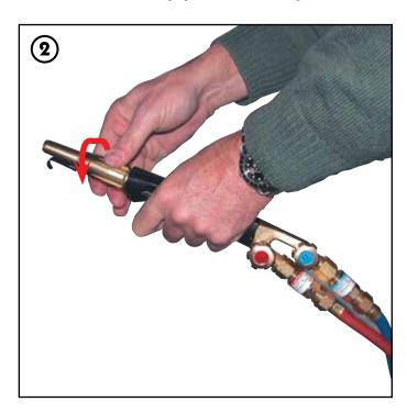
2. Fit mixer to the blowpipe handle and tighten by hand
