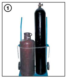
Secure both oxygen and acetylene cylinders on approved carry stand or trolley. (Not supplied)
