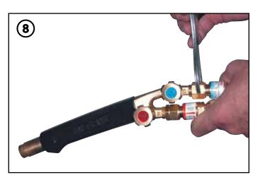
**8.** Attach **IBEDA** (AS4603) flash arrestors to blowpipe matching the respective colours and threads. Then attach the gas hose, which are colour coded and also thread oriented.
