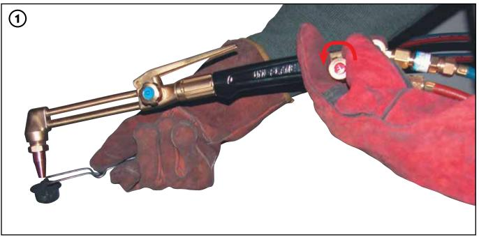
**4.** Open the oxygen heating control valve until a neutral flame is obtained with the cutting lever depressed. (Refer to flame adjustment setting chart fig A B C & D.)
