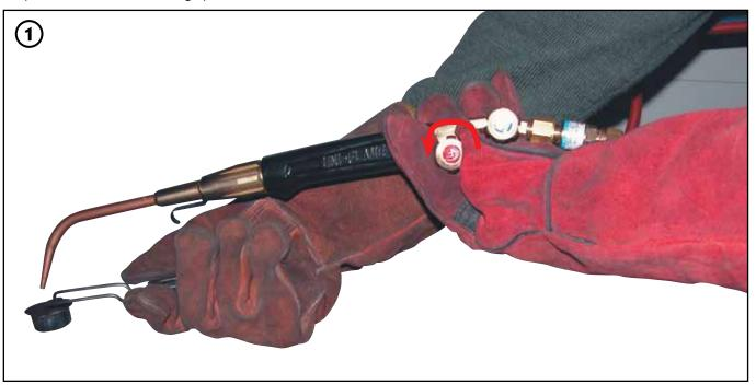
3. Open blowpipe oxygen control valve until a neutral flame is produced.
