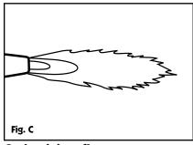
**Carburising flame** (obtained by having small excess acetylene). Ideal for hardening.
