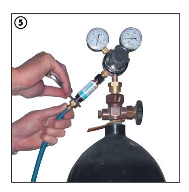
**5.** Attach gas hoses to flash arrestor on regulators using appropriate spanner. **Note: These are colour coded and thread orientated**
