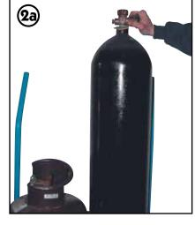
**2 - 2a.** Stand to one side and crack both oxygen and acetylene cylinders to clear any foreign material that may interfere with seating or clog orifices and threads.
