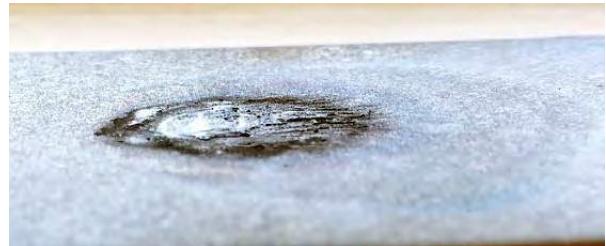
Spot weld removed
