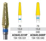
A new and optimised tungsten carbide cutter, hard coated with ZrN (zirconium nitride) for the reduction of plaster, denture acrylics, and preparation of composites. This new cutter gives you a smoother, faster operation and reduced heat generation due to less clogging. It also guarantees optimal surface quality with a longer cutter working life.
