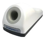
burners when waxing up. Simply place your waxing up instrument in and it is heated in the coil opening by induction in a matter of seconds, Requiring only a minimum energy consumption, the unit excludes carbon collecting on the waxing up instrument or in the sculpting wax. Even standard waxing up instruments can be used.
