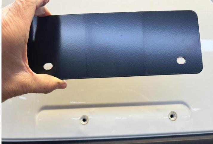
10. Peel the backing off the self adhesive tape on each plate.
