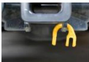
Step 1. Place the first half of the link through the hitch point on either side of the tow bar.
