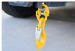
Step 5. Using a hammer, tap the pin through the collar until it emerges on the other side of the links.
