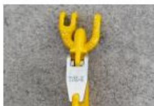
Step 2. Place the other half of the link through the eye of the hook.
