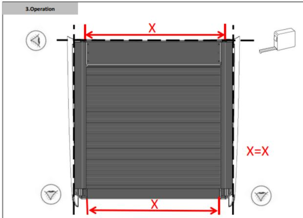
Make sure all the bolts are tightened; Close the roller and see if the roller is parallel on both sides as shown in pic. Measure if the distance are the same in front and rear(within 2mm difference is the best state).
