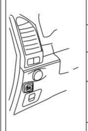
In order to facilitate user's operation, we offer an extra option with button control near driver's seat, so the user can easily control the cover.
