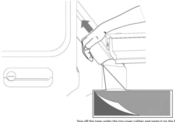
Tear off the tape under the top cover rubber and paste it on the front edge of the truck bed, then press down by hand to make it stick firmly.
