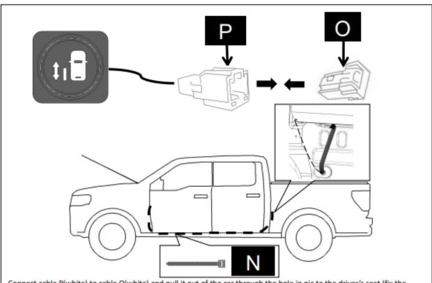
Connect cable P(white) to cable O(white) and pull it out of the car through the hole in pic to the driver's seat (fix the harness with N cable ties). Harness route need to avoid exhaust pipes, moving parts, vulnerable parts etc., thus to protect the vehicle as well as avoid harness damage.
