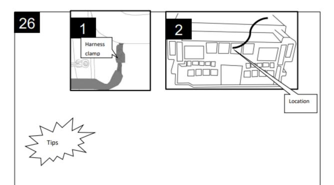
Open the trim panel on the driver's side (pillar A) with wire harness clips(pic 1) inside. Find the harness in pic 2, fasten original signal harness U(yellow wire) and original vehicle harness with U1T cable clip(pic 3). Refer to step 23(fix the harness with N cable ties), pull the harness out of the drain tube hole. Harness route need to avoid exhaust pipes, moving parts, vulnerable parts etc., thus to protect the vehicle as well as avoid harness damage.
