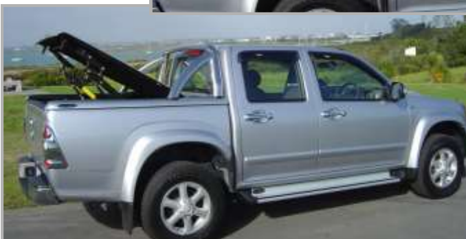
Custom Lid - hard lid (single or 2way open) (available with or without roll bar)
