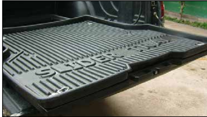
Bed Slide Light Duty -Load rated to 100kg # BS199
