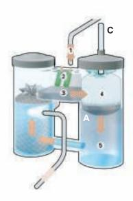
The condensate  ${\mathfrak O}$  passes through the silencer  ${\mathfrak O}$  into the expansion chamber  ${\mathfrak O}$ .
