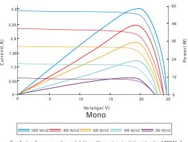
Excellent performance under weak light conditions: at an irradiation intensity of  $800W/m^2$  (AM 1.5, 25°C), 95.5% or higher of the STC efficiency( $1000W/m^2$ ) is achieved.
